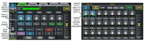
Figure 4.7d: Ch1-2 Linked, Aux1-2 also linked, both can be routed to Main mix
