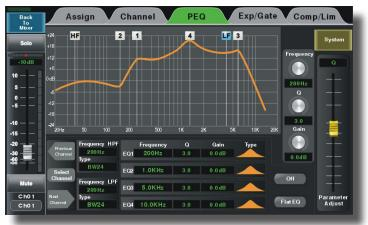
Figure 4.2: PEQ Parametric EQ Screen
